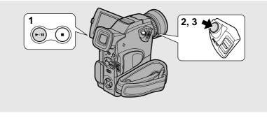
Record an image from a tape onto a memory card as still images. To automatically record multiple still images from a tape to a memory card, refer to "Copying Still Images from Tape to Memory Card" (
